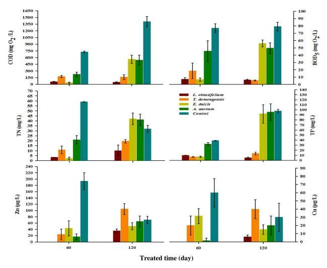
Figure 5 Changes of BOD<sub>5</sub>, COD, N, P, Zn and Cu following the treated time among treatments
