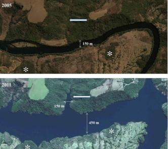
Figure 2. Satellite images before and after damming of the HET Amador Aguiar II, state of Minas Gerais. Arrows indicate habitat discontinuity after flooding. Notice also the dry forest patch brought near the reservoir shore (\*).
