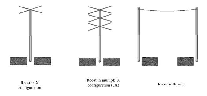
Figure 1. Types of artificial roosts that were used in this study. Hatched rectangles represent the seed collectors.
