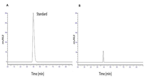
**Figure 5**. HPLC analysis. A – peak showing retention time of standard ethanol; B – ethanol yield after fermentation of saccharified waste office paper by *Alcaligenes faecalis* H1-1.
