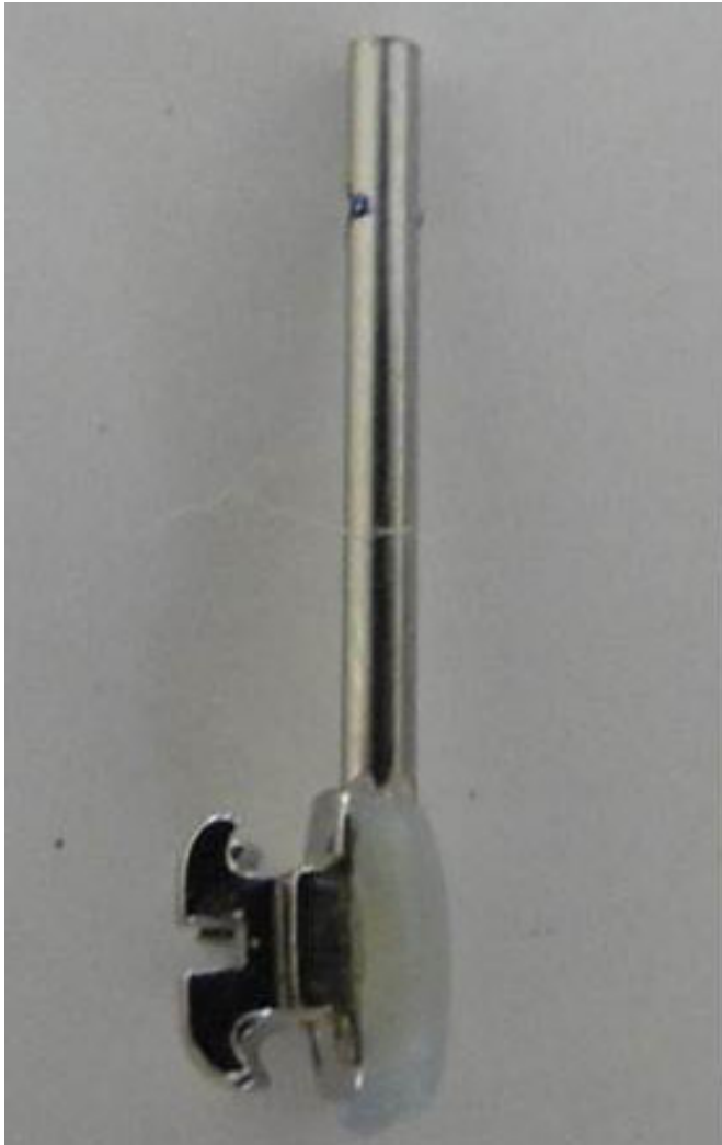
Fig. 2. Segment of an orthodontic wire (1.00 mm diameter x 14 mm long) fixed to the back of the Edgewise orthodontic test bracket.
