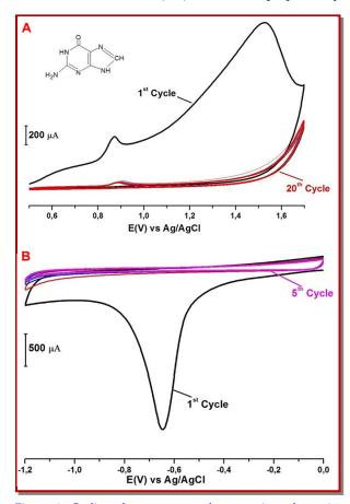
Figure 1: Cyclic voltammograms of preparation of guanine modified GC electrode, 1 mM aqueous solution of guanine was taken in 0.1 M  $H_2SO_4$  at 20 cycles with scan rate 0.1 V s<sup>-1</sup> (A). Cyclic voltammograms of reduction of guanine modified GC electrode, 0.1 M HCl was taken at 5 cycles with scan rate 0.1 V s<sup>-1</sup> (B)
