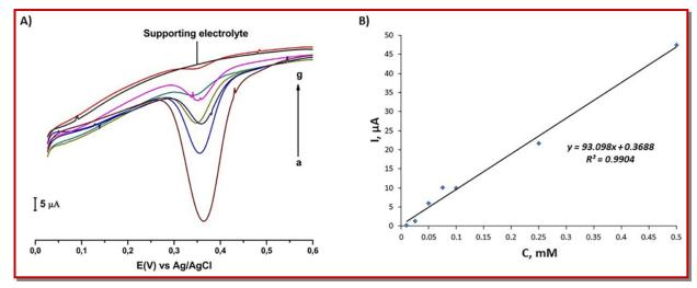
Figure 6: A) DPV curves of paracetamol on its concentration in the range of a)  $5.0 \times 10^{-4}$  M, b)  $2.5 \times 10^{-4}$  M, c)  $1.0 \times 10^{-4}$  M, d)  $7.5 \times 10^{-5}$  M, e)  $5.0 \times 10^{-5}$  M, f)  $2.5 \times 10^{-5}$  M, g)  $1.0 \times 10^{-5}$  M in BR buffer solution pH 5.0, and B) The plot of I<sub>pa</sub> versus concentration of paracetamol
