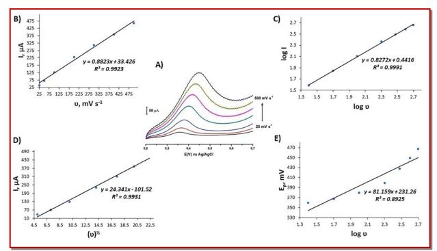
Figure 5: A) Impact of scan rate on 1.0 mM paracetamol in BR pH 5.00 at rGu/GC electrode from 20-500 mV s<sup>-1</sup>, B) shows the plot of the anodic peak current versus scan rate. C) Relation between log scan rate and log peak current. D) Calibration plot of the redox peak currents vs. square root of scan rate. E) Plot of variation of E<sub>p</sub>, mV versus log v, mV s<sup>-1</sup>
