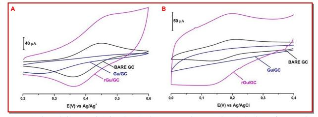
Figure 2: Overlaying the bare GC and rGu/GC electrode voltammograms at ferrocene and  $K_3Fe(CN)_6$ . A) 1 mM ferrocene redox probe solution vs. Ag/Ag<sup>+</sup> (10 mM) in CH<sub>3</sub>CN+ 0.1 M NBu<sub>4</sub>BF<sub>4</sub> using 0.1 V s<sup>-1</sup> scanning rate and B) 1 mM K<sub>3</sub>Fe(CN)<sub>6</sub> redox probe solution vs. Ag/AgCl/KCl(sat) reference electrode in BR buffer solution, pH 2.0 using 0.1 V s<sup>-1</sup> scanning rate
