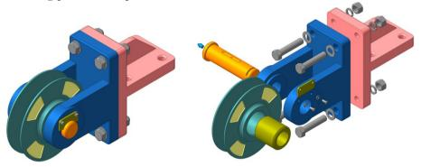
**Fig. 4.** The three-dimensional model of the block of the guide, created using COMPASS
