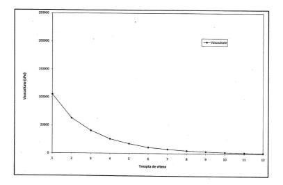
Figure 3: Viscosity variation depending on speed rate
