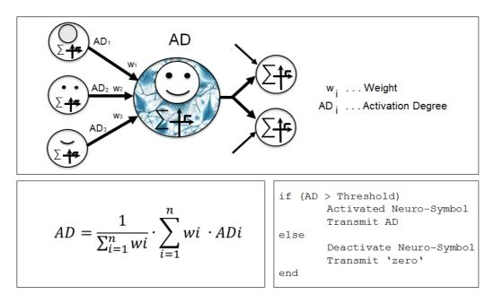
Figure 7. Function Principle of Neuro-Symbols
