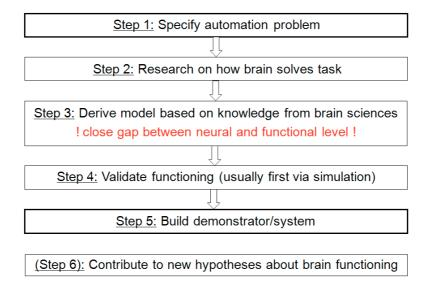
Figure 4. Methodology in the Field of Brain-Like Artificial Intelligence for Automation
