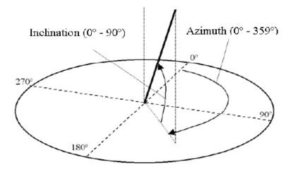
Figure 2. Azimuth and inclination angles of the pen respect to the plane of the graphic card GD-0405U from Wacom Graphire3 digitizing TabletPC
