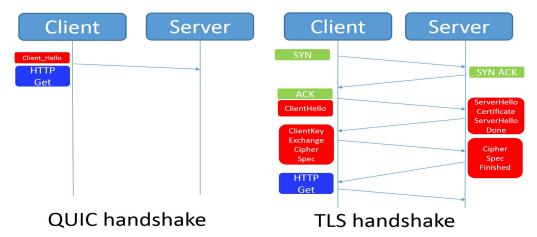
Figure 2. QUIC vs TLS handshake protocol
