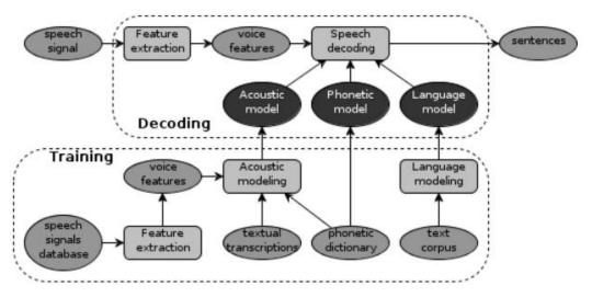
Figure 1. Main components of an ASR system (Cucu, PhD. Thesis, 2011)
