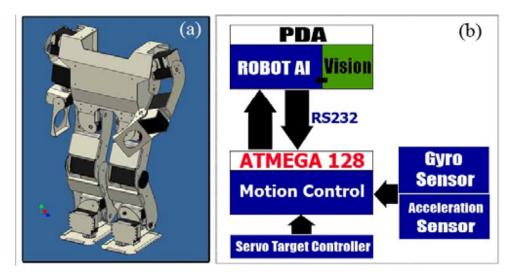
Figure 3. (a) Our Humanoid soccer robot, (b) Overview of the Control System
