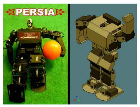
Figure 2. Mechanical construction of the PERSIA humanoid robots
