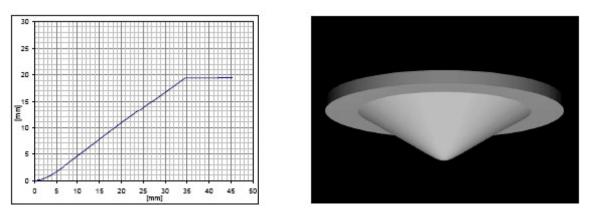
Figure 3 Profile of the overall mirror and the proposed mirror.
