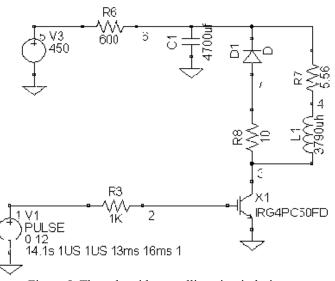
Figure 5. The solenoid controlling circuit design
