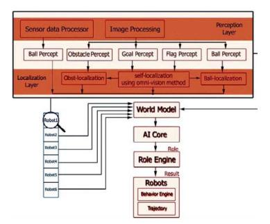
Figure 7. World model construction and artificial intelligent structure.
