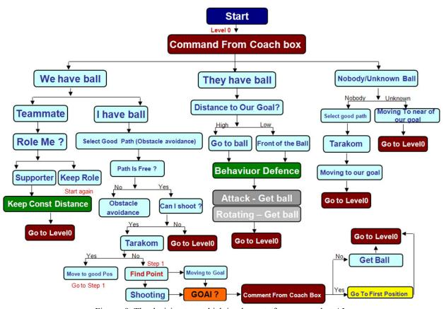
Figure 9. The decision tree which implements for soccer robot AI
