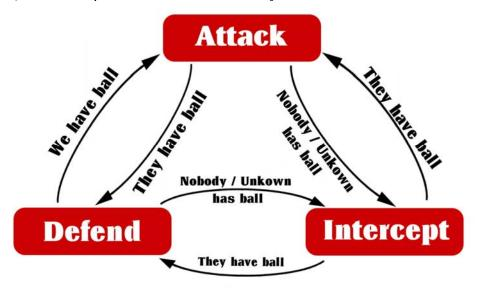
Figure 2. Finite state machine to determine the team strategy.
