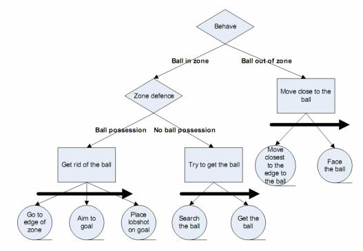
Figure 8. Example of a behavior tree: selector (diamond), sequence (rectangle), action (circle).
