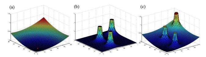
Figure 11. Potential at every point; it is highest in the obstacles and lowest at the goal. Elsewhere it is generally higher farther from the goal and near obstacles. [Image a describe the Goal force (Attractive potential to the goal) and image a describe the Obstacle force (Repulsive potential) and finally image c is Goal Force plus Obstacle force]
