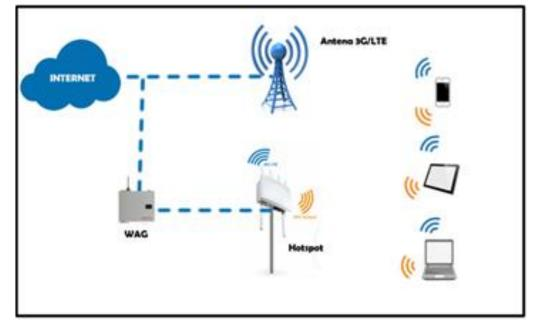
Fig. 1.Wi-Fi offloading network.
