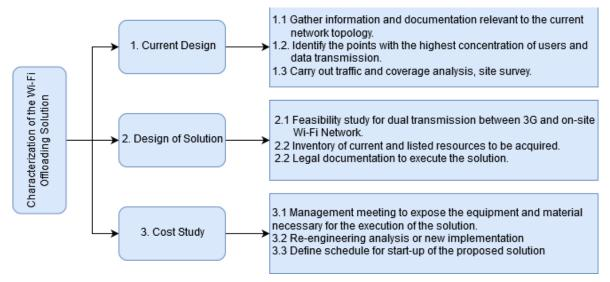
Fig. 2. Wi-Fi offloading solution characterization.
