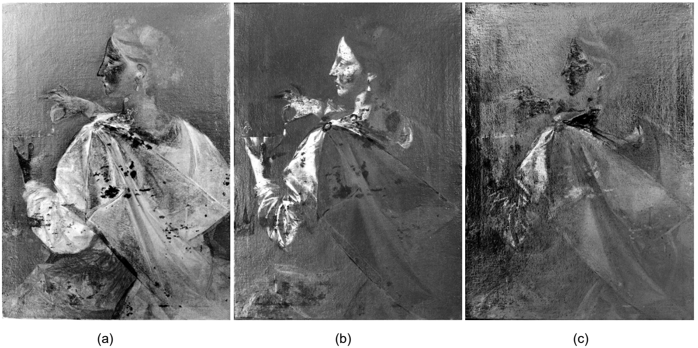
Fig.3 Some output channels of the FastICA algorithm from the multispectral set input. (a) Channel 1: here, the darkest regions correspond to the pictorial reintegration performed in 2019, especially in the face and shoulder. (b) Channel 3: the darkest regions in this ICA output correspond to the old pictorial reintegration. These regions are particularly visible on the profile of the forehead, nose and neck, the hand, and the red tunic. The numerous gaps also correspond to very dark pixels. (c) Channel 4: This output contains much information on the different restoration works; the gray levels represent the thickness of the color used. Black represents a dense color layer of color, whereas progressively light gray levels represent thinner color layers.
