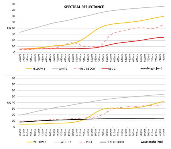
Fig. 9. Spectral reflectances of eight of the sixteen samples
