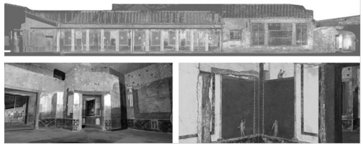
Fig. 5. Points cloud from the laser scansion of the peristyle and east dietae
