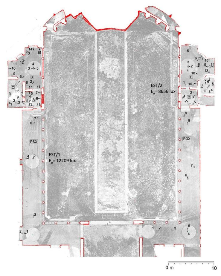
Fig. 6. Laser survey plan of the peristyle and dietae showing the irradiance measurement point
