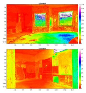
Fig. 12. Luminance maps in false colours referring to view 1 (above) and view 4 (below)
