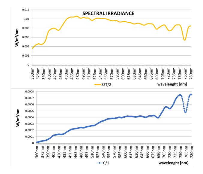
Fig. 7. Daylight spectral irradiance of the two extreme cases, EXT/2 (outdoor) and C/1 (indoor) regarding colour temperature.
