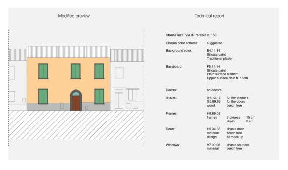
Fig. 4. Facade unit diagram and related technical report.
