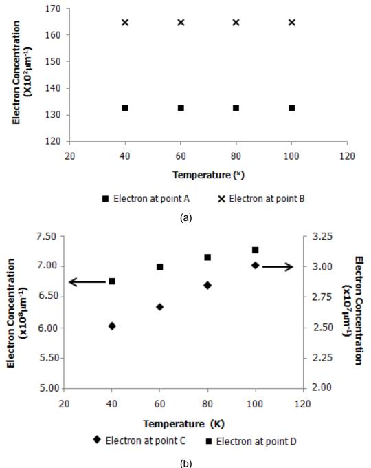
Figure 3. The curve of electron concentration as function of temperature at point A, and B (a) and also for point C, and D (b)
