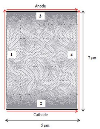
Figure 1. GaAs semiconductor crystal geometry which has been divided into triangular-shaped elements
