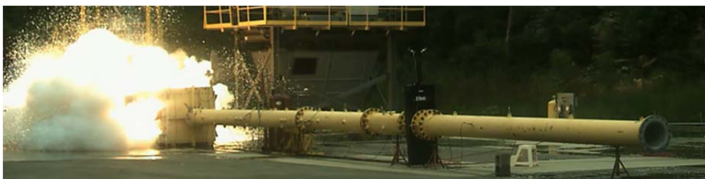
Figure 4: Mechanical explosion isolation of an aluminium dust ( K_{St} = 450 \text{ bar m/s} ) deflagration initiated in a 5\text{-m}^3 vented vessel (Taveau, 2017)
