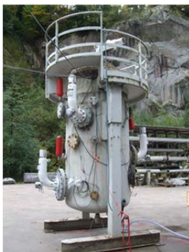
Figure 3: 4.4 m 3 vessel (FSA) used for the suppression tests and comparison of the explosion pressure curves from 1-m 3 and 4.4-m 3 suppression tests with 500 g/m 3 of aluminum dust (Taveau et al., 2015)
