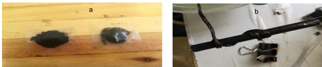
Figure 6a: Membrane fouling on the anode chamber side.
