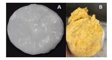
Figure 1 Membrane of purified BC (A) and sugarcane bagasse (SCR) (B)
