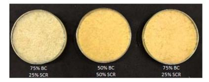
Figure 2 Paper samples prepared with varied BC and SCR composition
