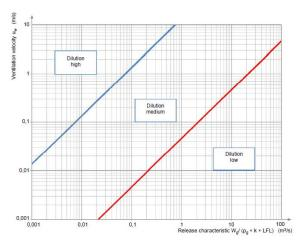
Figure 2: Dilution degree assessment (IEC EN 60079-10-1)
