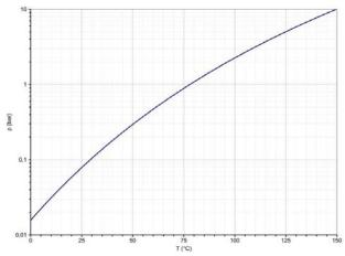
Figure 1: Bioethanol vapour pressure
