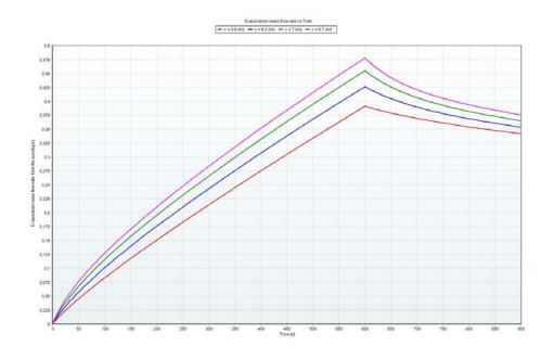
Figure 4: Trend of bioethanol evaporation rate
