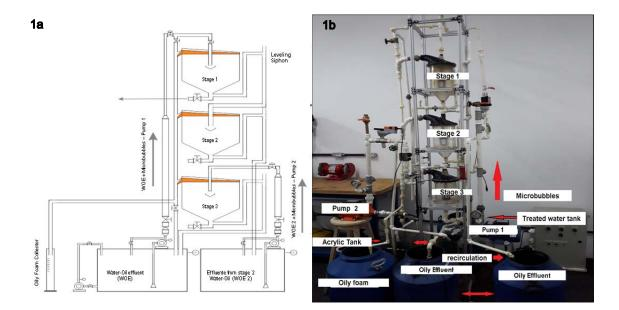
Figure 1 - Bank-scale induced saturation tower. (1a) indicates the flowchart and (1b) actual prototype photo
