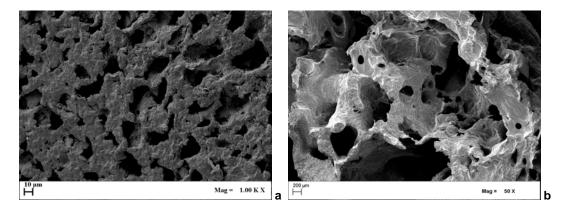
Figure 3: SEM images of a) PVDF-HFP and b) PVL50.
