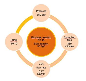
Figure 2. Optimized operational conditions adopted for extracting astaxanthin from Haematococcus pluvialis via supercritical CO<sub>2</sub> operation (Molino et al., 2018b, c).
