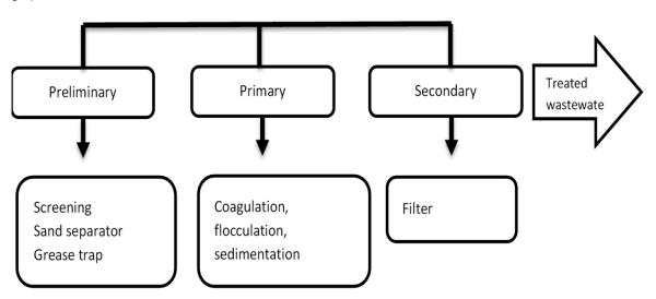
Figure 1: Process 1 Physical-chemical treatment
