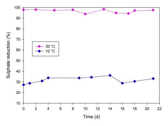
Figure 1: Temperature effect on sulphate reduction at pH 6 and HRT of 4.5 d.
