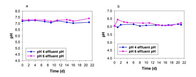
Figure 3: Effluent pH 4 and 6 at (a) 20 °C and HRT of 7 d and (b) 10 °C and HRT of 4.5 d.
