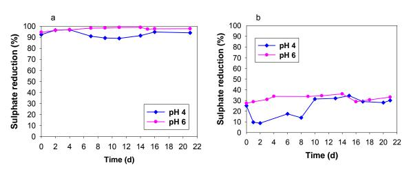
Figure 2: pH effect on sulphate reduction at (a) 20 °C and HRT of 7 d and (b) 10 °C and HRT of 4.5 d.
