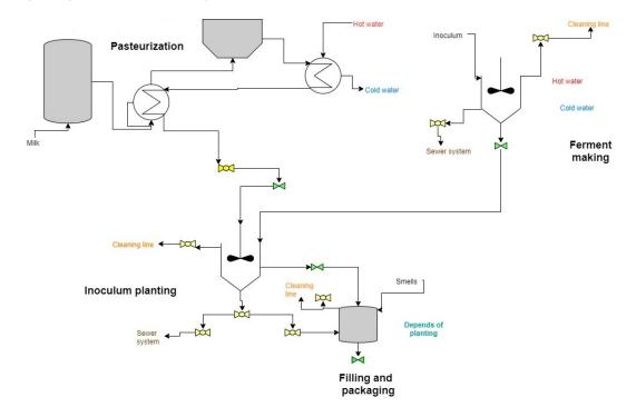
Figure 1: P&ID Process Pasteurization and Mixing
