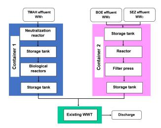
Figure 1: Block scheme of the pilot plant
