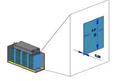
Figure 2. Fixing the electrodes inside the oxyhydrogen gas generating device
