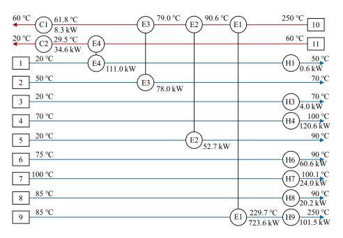
Figure 2: Grid diagram of the HEN after retrofitting using constrained PSO
