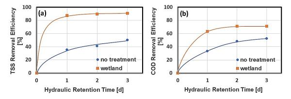
Figure 6: Removal efficiency of (a) TSS and (b) COD in wetland effluent and in control tank
