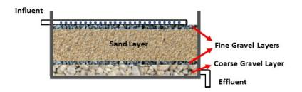
Figure 3: Schematic diagram of SSF wetland in this study
