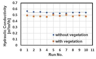
Figure 4: Hydraulic conductivity test results of wetland media
