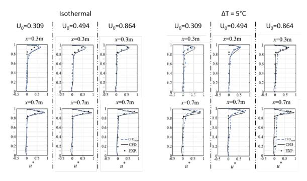
Figure 2: Comparison of CFD<sub>new</sub> (isothermal and  $\Delta T_{inlet} = 5 \text{ °C}$ ) simulations of normalized x-velocities ( $u^* = u_x/u_0$ ) with Deng et al. (2018) simulated data and experimental results.
