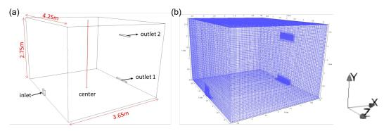
Figure 3: (a) Geometry and (b) mesh of simulated room with fresh air vent height = 0.05 m.
