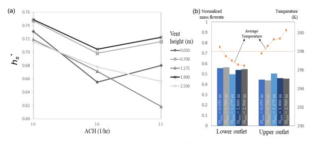
Figure 6: Comparison of (a) normalized sensible heat rate,  $h_s^*$  with different ACHs and vent heights; (b) normalized mass flowrate and temperature of upper and lower outlet for ACH = 10
