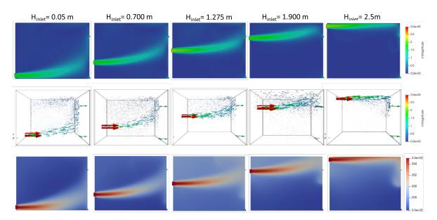
Figure 4: Comparison of velocity contour, velocity vector, and temperature profile of air at the xy-plane for different vent heights obtained using numerical simulations for ACH = 10.
