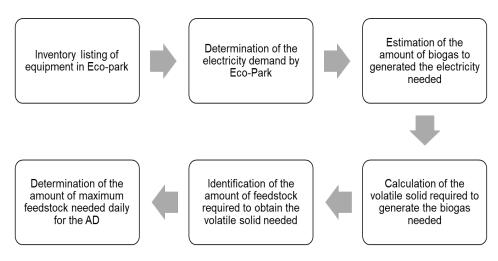
Figure 2: Process flow in designing the pilot-scale AD for Eco-park UTM
