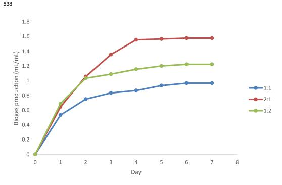
Figure 3: Daily biogas production(mL of biogas/mL of feed) for three samples with different ratios of FVW and POME
