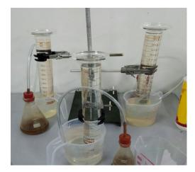
Figure 1: Experimental setup for lab-scale AD
