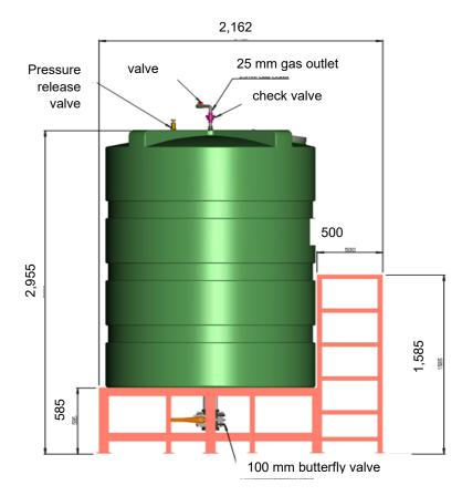
Figure 5: The design of the pilot-scale AD for Eco-park UTM
