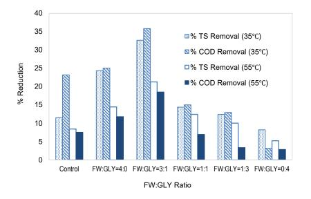
Figure 3: Reduction of TS and COD with various ratios of food waste to cruse glycerol at 35 °C and 55 °C
