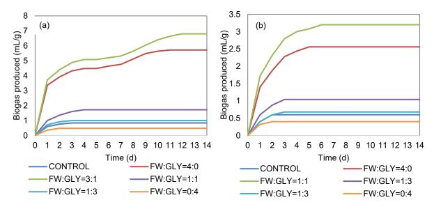
Figure 2: Cumulative biogas production during the batch co-anaerobic digestion with various ratios of food waste to crude glycerol at (a) 35 °C, and (b) 55 °C
