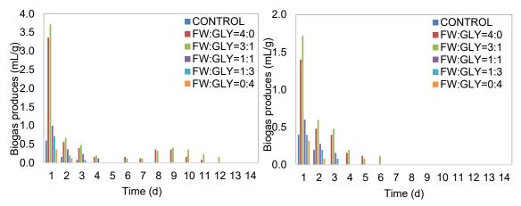
Figure 1: Daily biogas production during the batch co-anaerobic digestion with various ratios of food waste to crude glycerol at (a) 35 °C, and (b) 55 °C
