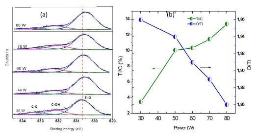
Figure 3: XPS O 1s core peak of decorated graphenic powder(a) and variations of Ti/sp<sup>2</sup>C and O/Ti atomic ratio (oxide stoichiometry in function of the applied RF power for sputtering (b).
