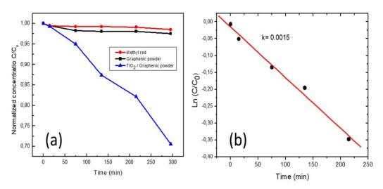
Figure 4: (a) Normalized dye concentration  $(C/C_0)$  time variation under solar light exposure of decorated graphenic carbon powder with  $TiO_2$  nanoparticles at 80 W, uncoated powder and methyl red (b)  $Ln(C/C_0)$  - Time plot for the determination of the rate constant as the slope of the data linear fit, for the powder decorated at 80 W.
