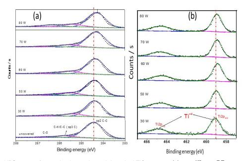
Figure 2: XPS spectra for graphenic powder and deposited  $TiO_2$  nanoparticles at different RF power values (a) C 1s core levels with marked positions of the C-C (sp2) bond (b) Ti 2p core level spectra.
