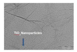
Figure 1: TEM image of deposited TiO2 nanoparticles onto the graphenic sheets composing the powder.
