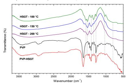
Figure 1: FTIR spectra of HSGT samples heated for 1 h at 100, 150 or 200 °C, electrospun PVP and composite PVP-HSGT mats (dotted lines indicate the main bands of TiO<sub>2</sub>-acac).
