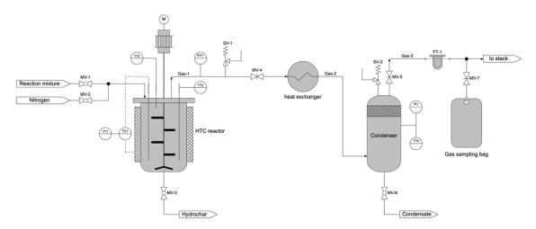
Figure 1: Schematic illustration of the bench-scale HTC apparatus
