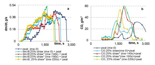
Figure 3: Effect of the increasing irradiation time for wheat straw pellets on the weight loss at the thermal decomposition of the 25% straw (MW)\*+peat mixture (a) and on the yield of CO (b)
