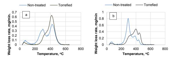
Figure 6: DTG curves (in air) of non-treated and torrefied (300 °C) peat (a), and wheat straw (b) samples
