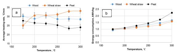
Figure 1: Average rate of MW assisted heating of biomass (a) and specific electric energy consumption (b) depending on the torrefaction temperature
