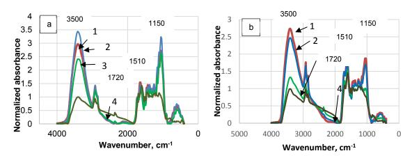
Figure 5: FTIR spectra of wheat straw (a), and peat (b) normalized at 1510 cm<sup>-1</sup>: non-treated (1), and torrefied at the temperatures: 200 °C (2); 250 °C (3), 300 °C (4)
