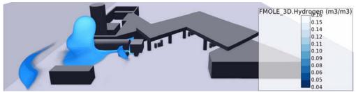
Figure 2: 3D plot of the H<sub>2</sub> flammable cloud at 76 s for the vertical upward release (simulation nr. 33).
