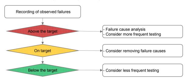
Figure 2: An example on how to use a performance indicator (e.g. observed number of DU failures) for verifying SIL requirements in the operational phase. Adapted from (Hauge et al., 2008).
