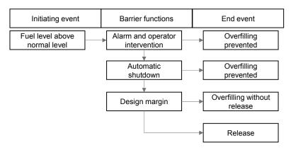
Figure 3. A barrier block diagram for release from the tank due to overfilling.
