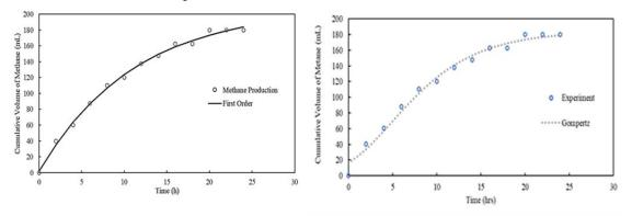
Figure 3: Kinetics Models Fitting for (a) First Order Kinetic Model (b) simplified Gompertz Model
