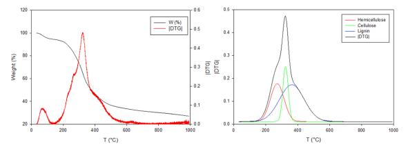
Figure 3: Weight percentage and DTG curves as a function of temperature, TG/DSC analysis, 10 °C/min,  $N_2$  flow (left), and deconvolution through Fraser-Suzuki equation of DTG curve (right).
