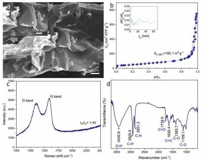
Figure 1: SEM images (a), adsorption-desorption isotherms with BJH plot inset (b), Raman analysis (c), and FTIR analysis (d) of graphene-OH.
