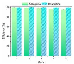
Figure 5: Adsorption-desorption of AMX onto and from graphene-OH at  $C_o = 80$  mg  $L^{-1}$ , S/L = 10, pH = 5, and T = 25 °C.
