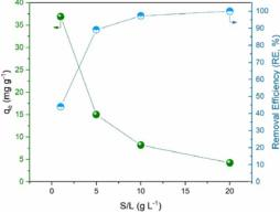
Figure 4: Effect of adsorbent dosage to the adsorption of AMX onto graphene-OH at varied solid to liquid (S/L) ratio,  $C_0 = 40 \text{ mg L}^{-1}$ , pH = 7, and  $T = 25 \text{ }^{\circ}\text{C}$ .
