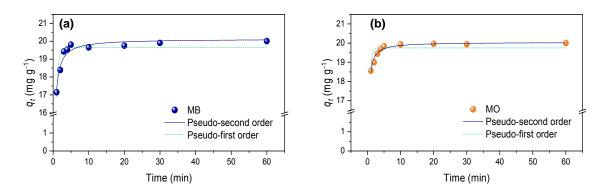
Figure 3: Time profile and kinetic model fitting of (a) MB and (b) MO adsorption in CNT at Co =  $20 \text{ mgL}^{-1}$ , pH = 7, S/L ratio =  $0.1 \text{ gL}^{-1}$ , V = 25 mL, and T =  $25 ^{\circ}$ C.
