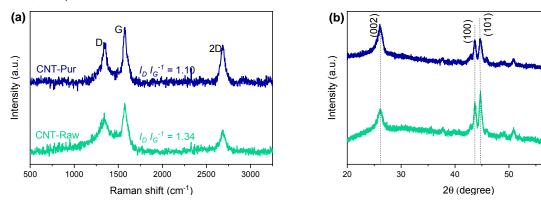
Figure 2: (a) XRD and (b) Raman spectra of raw and purified CNT from PWO
