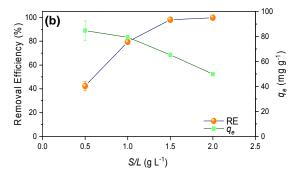
Figure 5: Effect of dosage for (a) MB and (b) MO in CNT at C<sub>o</sub> = 100 mgL<sup>-1</sup>, pH = 7.0, and T = 25 °C
