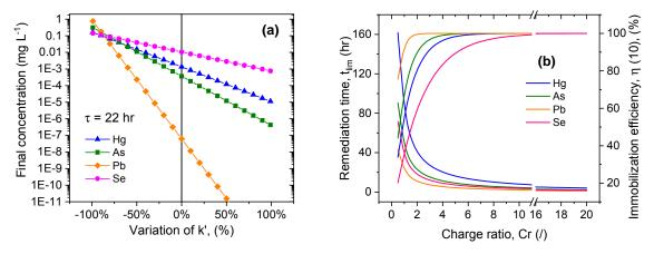
Figure 3. Sensitivity of simulated HMs concentrations in the leachate after 22 hours milling to the variation of the parameter k' (a); simulated effect of Cr change on the remediation time and immobilization efficiency after 10 hours of mechanical treatment (b).
