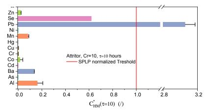
Figure 4. Effect of 10-h ball milling by the attritor using  $C_R$ =10 on the normalized concentrations of leached HMs
