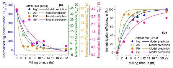
Figure 2. Time evolution of normalized HM concentrations (a) and immobilization efficiency (b) using the
