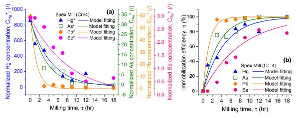
Figure 1. Time evolution of normalized HM concentrations (a) and immobilization efficiency (b) using the SPEX
