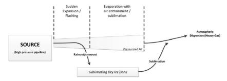
Figure 1: Typical source term components within a CO2 release framework (Mocellin et al., 2016a).
